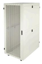
The second rack was the Environ SR 800mm x 1000mm Server Rack which provided even more features including a vented wave design mesh front door and a vented wardrobe double mesh back door for maximum ventilation of around 70%. There was easy access with removeable side panels and with a load capacity of 1300kg it was more than capable to house all of the servers and switches.
